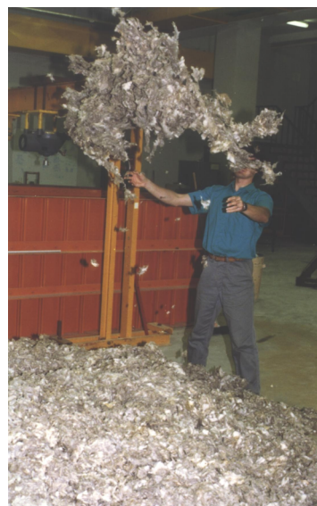
Figure 4. Manual blending of the wool to achieve a homogenous mix.
