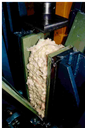
Figure 2. Wool in lubricated, retracted chamber (before pressing).
